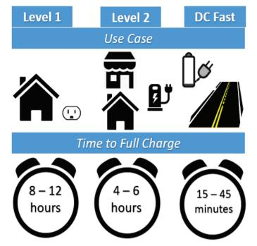
Figure 3-2: Charging Technologies for Electric Vehicles
