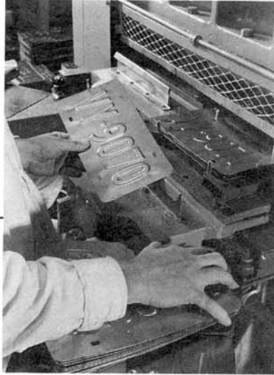
Raw plates are placed in a rimmer press where the edges are crimped and "Texas" and date are stamped on bottom.
