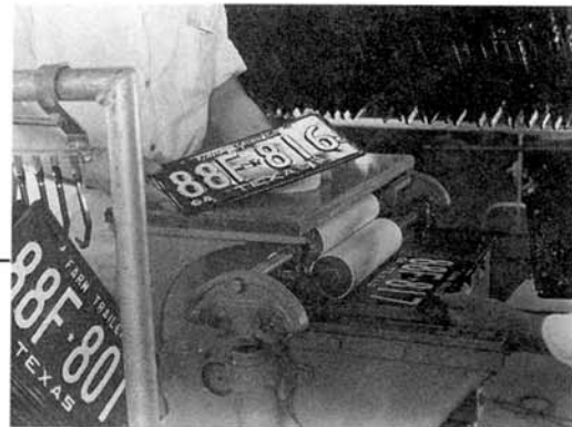
Raised numbers and letters on the plates are painted white in this inking machine.
